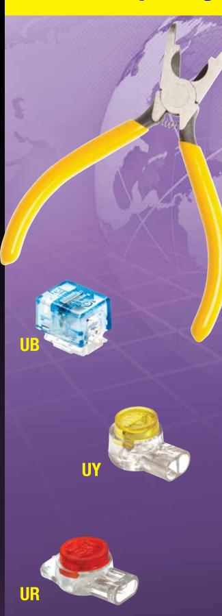
These quality pliers are designed to crimp **UG**, **UR**, **UB** and **UY** style connectors manufactured by 3M and others. Pliers are designed and manufactured in accordance with Bell Specifications. They feature a built-in side-cutter and coil spring. The built-in stop prevents damage to connectors. Vinyl-dipped handles.
